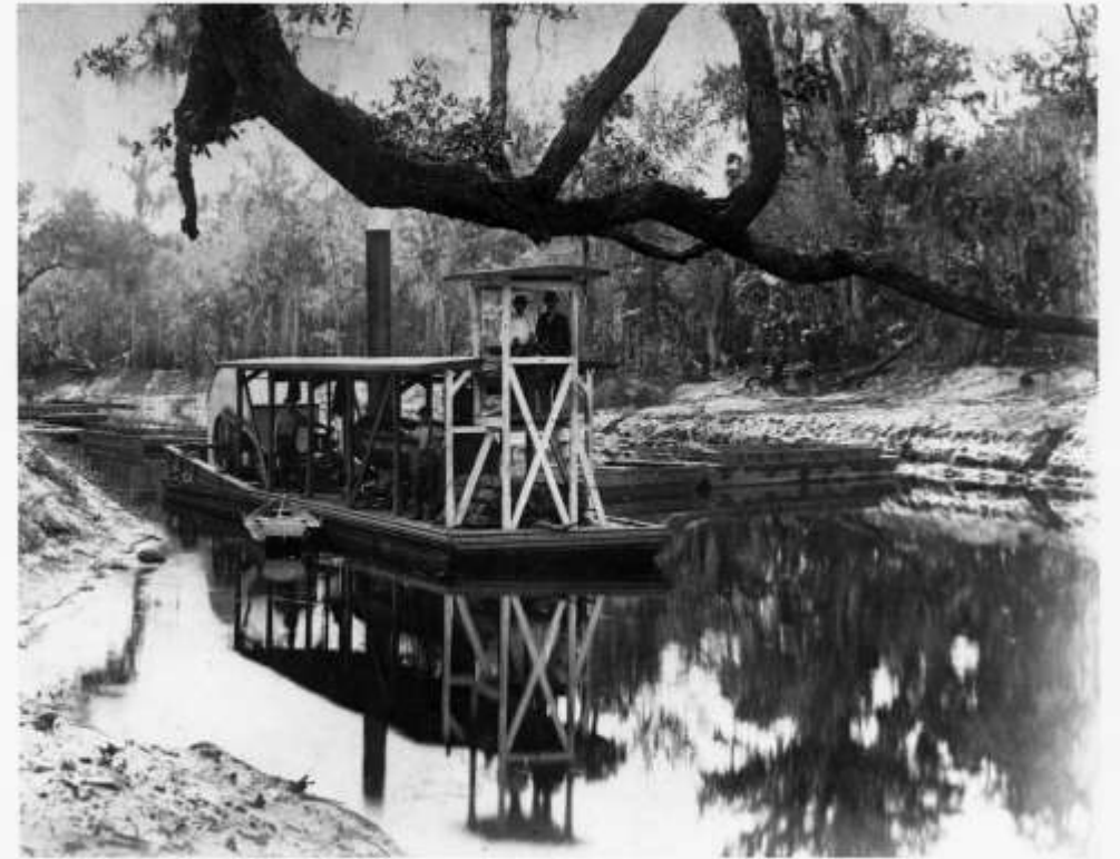
A makeshift tugboat, Little Steamer No. 1, consisting of a boiler, engine and pilot's deck strapped to a flat-top barge, is shown here towing empty phosphate barges back up the Peace River, ca. 1902
